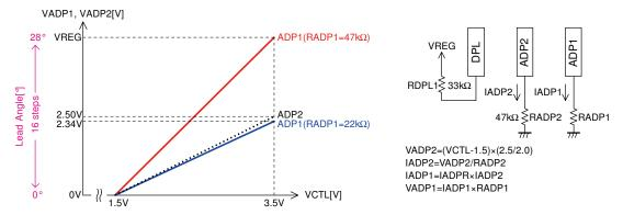
2. The ADP2 pin rise can be halted (a limit on the lead angle adjustment can be set by means of the CTL voltage) by setting DPL (pin 25).
