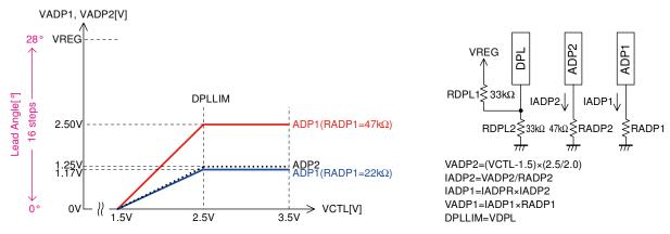
3. The offset and slope can be adjusted as desired by setting RADP1 and RADP12 of ADP1 (pin 30). (It is also possible to set a limit on the lead angle adjustment by means of the CTL voltage by setting DPL.)
