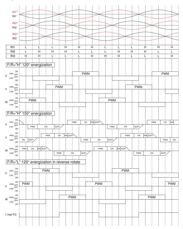
The energization is switched to  $120^\circ$  wher 1 Hall FG frequency is 3.6Hz (typ) or lower A direction of rotation is detected from Hall signal according to F/R pin input If the motor rotates in reverse against F/R pin input  $120^\circ$  energization is maintained forcibly
