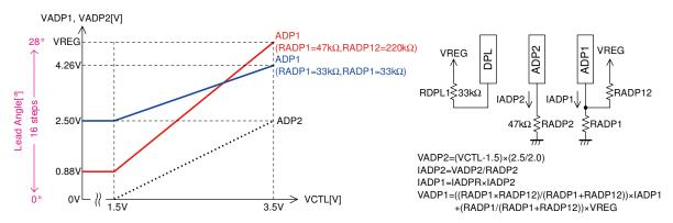
4. The rising voltage of ADP1 can be adjusted using the settings of RADP21 and RADP22 of ADP2 (pin 28). However, they must be set in such a way that the ADP2 voltage does not exceed 1V when V<sub>CTL</sub> is lower than 1.5V.
