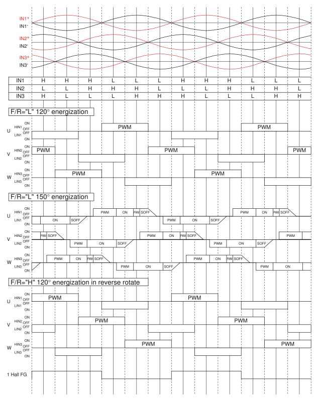
The energization is switched to 120° wher 1 Hall FG frequency is 3.6Hz (typ) or lower A direction of rotation is detected from Hall signal according to F/R pin input If the motor rotates in reverse against F/R pin input 120° energization is maintained forcibly
