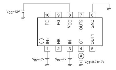
CT pin charge/discharge voltage (VCT)
