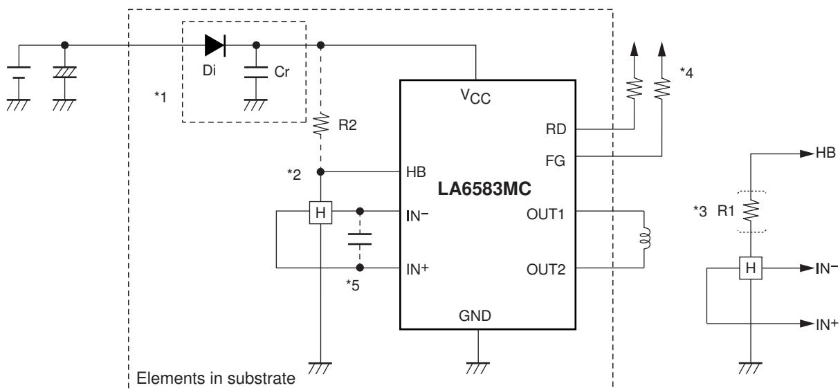
\*1: When Di to prevent breakdown in case of reverse connection is used, it is necessary to insert a capacitor Cr to secure the regenerative current route. Similarly, Cr is necessary to enhance the reliability when there is no capacitor near the fan power line.
