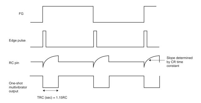
By changing the pulse width as determined by the CR time constant, the VCTL versus rotational speed slope can be adjusted as shown in the speed control diagram in the previous section.
