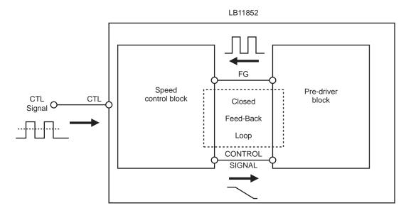
The operation inside the IC is as flows. pulse signals are created from the edges of the FG signals as shown in the figure below, and using these signals as a reference, waveforms with a pulse width determined by the CR time constant are generated using a one-shot multivibrator. These pulse waveforms are then integrated to control the duty ratio of the pre-driver output as the control voltage.
