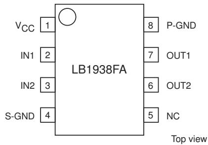
S-GND: GND for the control system
