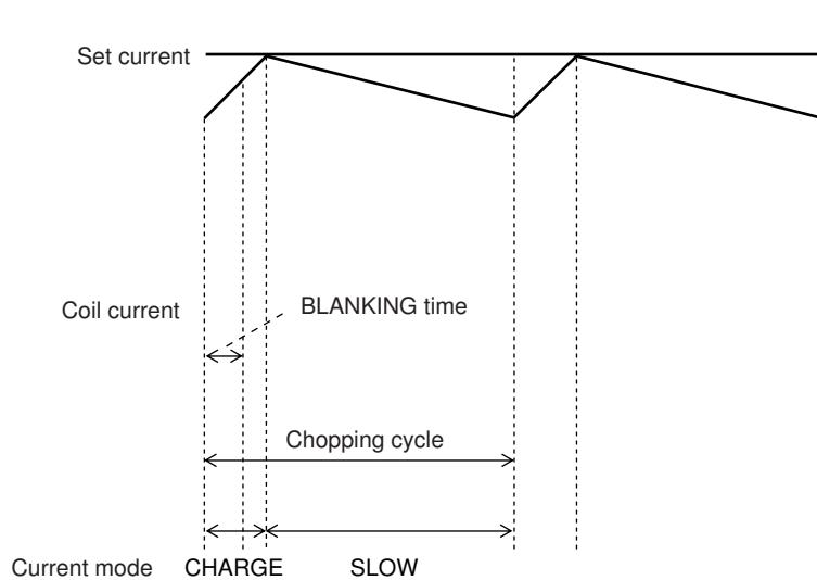
Based on the voltage input to the VREF pin and the resistance connected between RF and GND, the output current that is subject to the constant-current control is set using the calculation formula below :
