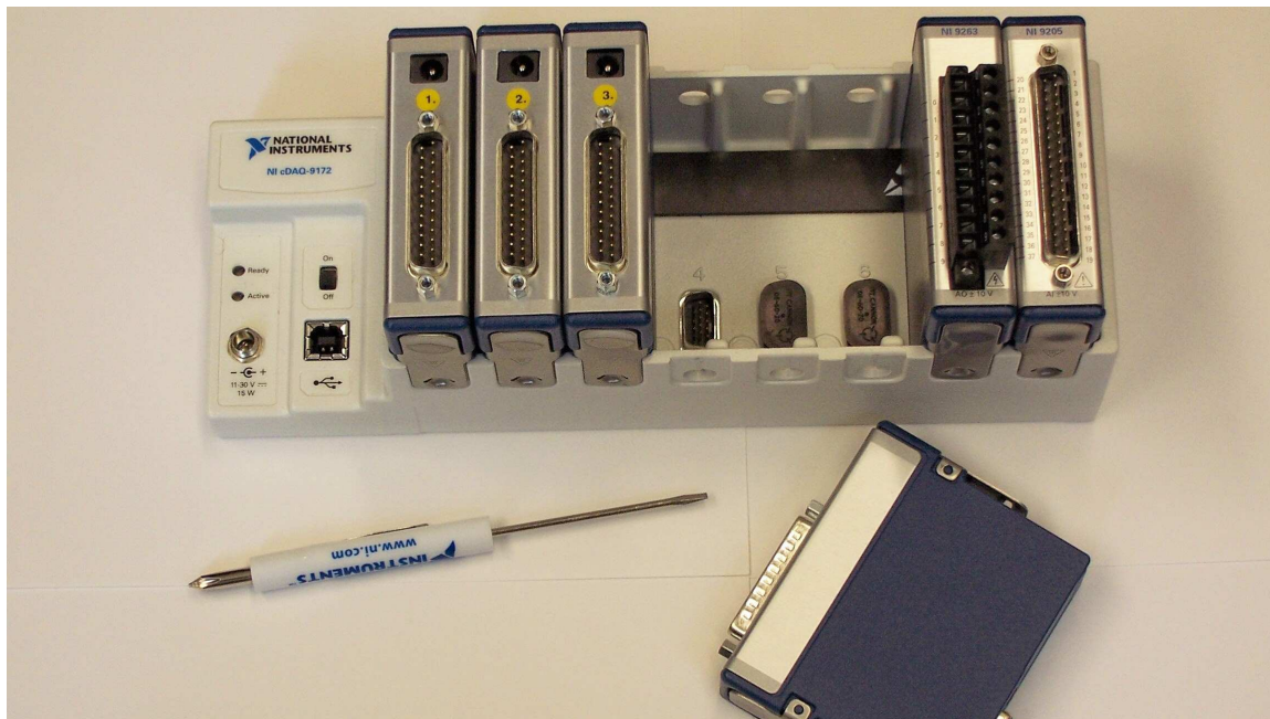
Figure 1: MBK-600 MultiCal System Shown with MB-121, MB-122 and MB-123 installed. MB-124 is shown in the foreground
