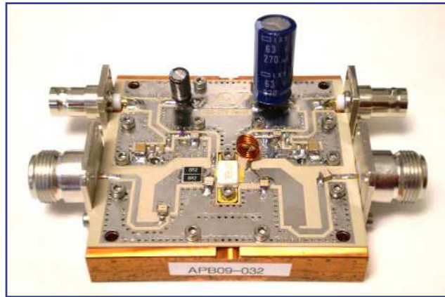
Figure 12 - Photograph of 500-1000MHz broadband application circuit for NPT1010
