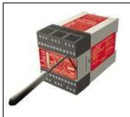
Figure 7. To remove the Module's terminal strips, insert a small screwdriver blade into each of the four slots at the top and bottom of the front cover.
