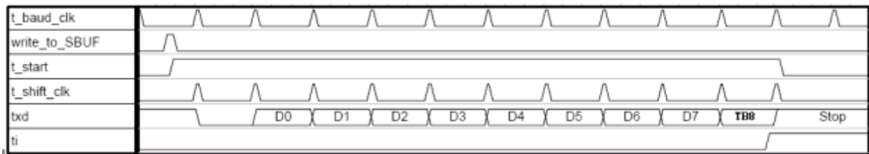
Fig. 9-5: Transmit modes 2 and 3 for Serial 0
