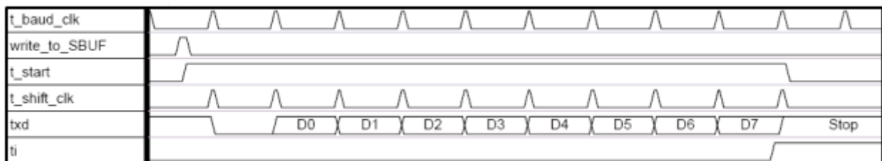
Fig. 9-3: Transmit mode 0 for Serial 0
