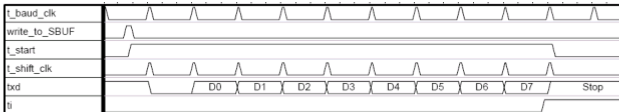
Fig. 9-9: Transmit mode B for Serial 1
