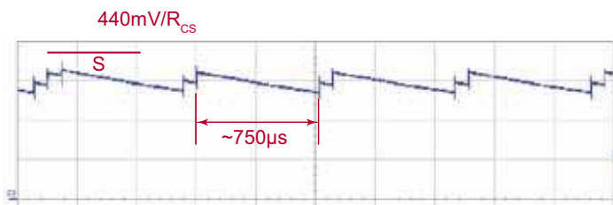
Fig.2. Short-circuit inductor current.
