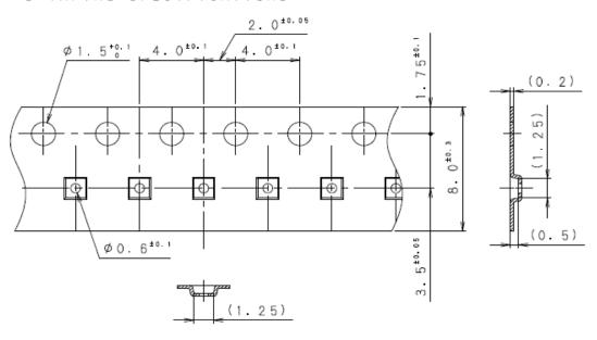
NOTE)1. THE R MEASUREMENT WITHOUT INDICATION IS ASSUMED TO BE O. 3 mm WAX. GENERAL TOLERANCE: ± O. 2
