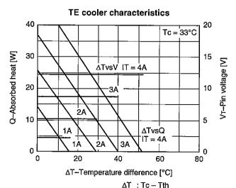
$\begin{array}{ll} \Delta T & : Tc - Tth \\ Tth & : Thermistor\ temperature \\ Tc & : Case\ temperature \end{array}$
