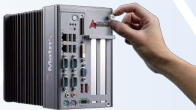
1. Undo the thumbscrew by hand
