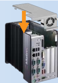
3. Replace it by plugging the hot-pluggable fan module cover into the fan connector on CPU board
