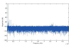
Typical values are measured using 1 MHz sine wave input at 100 MS/s with amplitude at -1dB of full scale on a  $\pm$  2V range. Acquired data lengths are in 64k points, calculated with Hanning window FFT.
