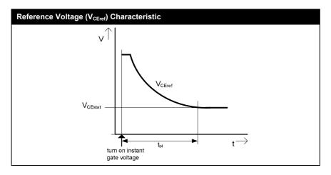
After  $t_{bl}$  has passed, the  $V_{CE}$  monitoring will be triggered as soon as  $V_{CEsat} > V_{CEref}$  and will turn off the IGBT. The error memory will be set, and the output PRIM\_nERROR\_OUT changes to the HIGH state. Possible failure modes are shows in the following pictures.
