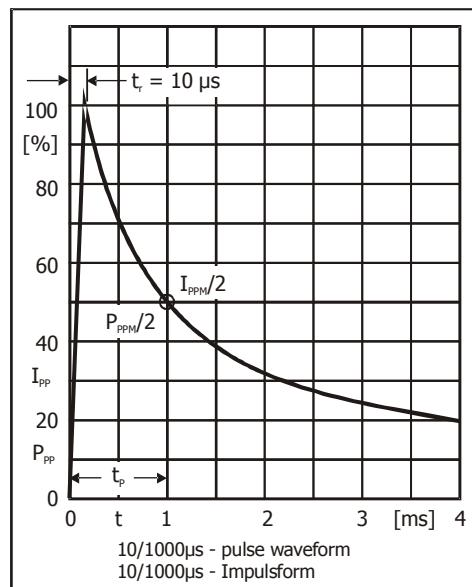
10/1000μs - pulse waveform
