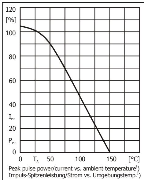
Peak pulse power/current vs. ambient temperature<sup>1)</sup>
