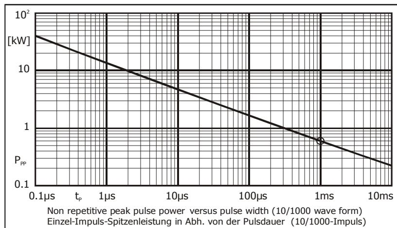
Non repetitive peak pulse power versus pulse width (10/1000 wave form)
