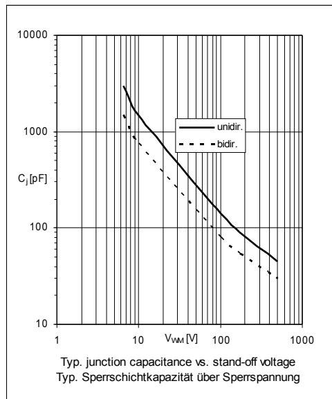
Typ. junction capacitance vs. stand-off voltage
