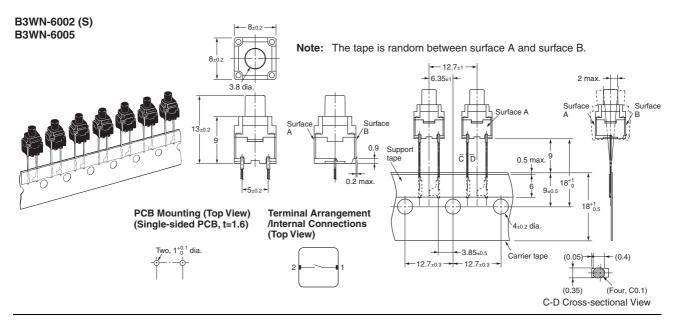
Note: Unless otherwise specified, a tolerance of  $\pm 0.4$  mm applies to all dimensions. No terminal numbers are indicated on the Switches.
