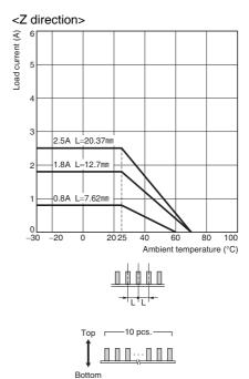
• Thirty Relays are soldered to the PCB at each given spacing.
