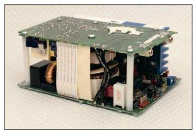
The CE300AHX, CE300BHX, and CE300CHX power supplies are designed to run Mercury-Xenon arc lamps in a constant-power mode.
