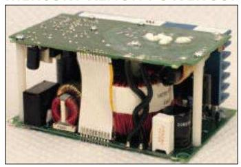
The CE200AHX, CE200BHX, and CE200CHX power supplies are designed to run mercury-xenon arc lamps in a constant-current mode.
