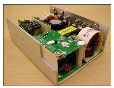
The CEP301AHG, CEP301BHG, CEP301CHG, CEP301AMH, CEP301BMH, and CEP301CMH power supplies are designed to run mercury and metal halide arc lamps in a constant-power mode or constant current mode.
