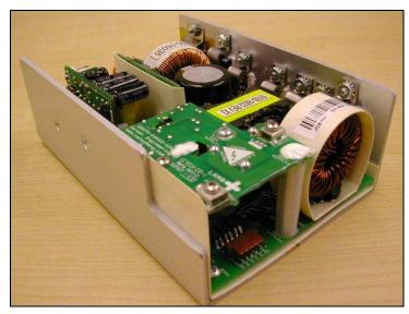
The CEP301AXE, CEP301BXE, CEP301CXE, CEP301AHX, CEP301BHX, and CEP301CHX power supplies are designed to run Xenon arc lamps in a constant-power mode or constant current mode.
