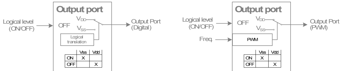
Figure 8. Output logic on the digital and PWM ports
