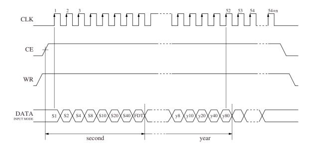
Data is input when WR is HIGH and CE is HIGH.
