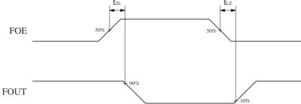
Note that FOE and FSEL do not have chatter elimination circuits. Consequently, switching either FOE or FSEL during 32kHz mode operation may generate chatter noise on the FOUT output. Also, note that the 1Hz and 32kHz oscillators are not synchronized to each other, so switching intervals shortens the duty cycle. Accordingly, a wait time (≥ chattering time + output frequency period) should be incorporated when switching intervals.
