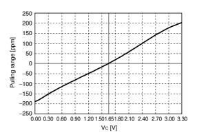
$V_{DD}$  = 3.3V,  $f_{OUT}$  = 27MHz, Ta = R.T.
