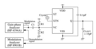
$C1=33\mu F,\,R1=R2=1M\Omega$  VC modulation signal: 100Hz to 100kHz, 0 to  $V_{DD}p\text{-}p$
