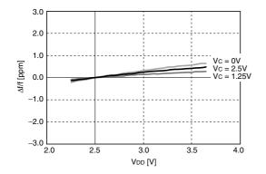
$f_{OUT}$  = 27MHz,  $\pm$  0ppm at  $V_{DD}$  = 2.5V, Ta = R.T.
