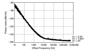
$V_{DD}$  = 2.5V,  $f_{OUT}$  = 27MHz, Ta = R.T.
