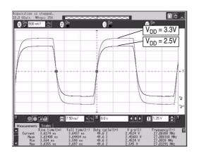
$$\begin{split} V_{DD} = 2.5 \text{V, } 3.3 \text{V, } f_{OUT} = 27 \text{MHz, } V_{C} = 0.5 V_{DD}, \\ C_{LOUT} = 15 \text{pF, } \text{Ta} = \text{R.T.} \end{split}$$
