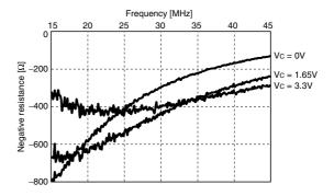
$V_{DD}$  = 3.3V, C0 = 2pF, Ta = R.T.
