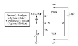
Note. "C0" value is set, concerning the actual crystal characteristics connected between XT and XTN. The data is measured with Agilent 4396B using NPC's original measurement jig. The values may vary with measurement jig and conditions.
