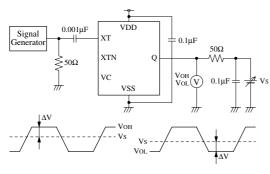
$V_S$  adjusted such that  $\Delta V$  =  $50 \times I_{OH}$ .
