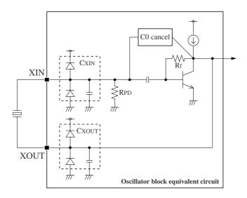
The 5037A1/B×/C×/D×(T)/E× oscillator circuit has a C0 cancel circuit built-in to improve the oscillator margin. If power is applied when there is an open circuit between XIN and XOUT, self oscillation may occur, which is not abnormal. Users should confirm that the oscillator operates normally when a crystal unit is connected.
