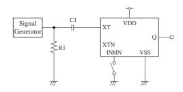
2Vp-p, 10MHz sine wave input signal
