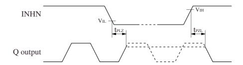
INHN input waveform  $tr = tf \le 10ns$
