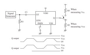
2Vp-p, 10MHz sine wave input signal
