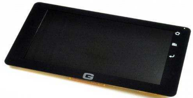
7" Display with Multi-touch Capacitive Screen
