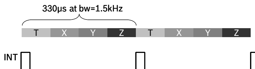
Figure 35: Explanation of data ready interrupt: For a bandwidth of e.g. 1.5 kHz the data refresh cycle takes 330µs to update all data registers. After the final conversion of z-axis the INT pad will be set high. New data can be read out via interface (recommendation: read out within 20µs after interrupt is high during the conversion of the next temperature value). The interrupt resets automatically after read out.
