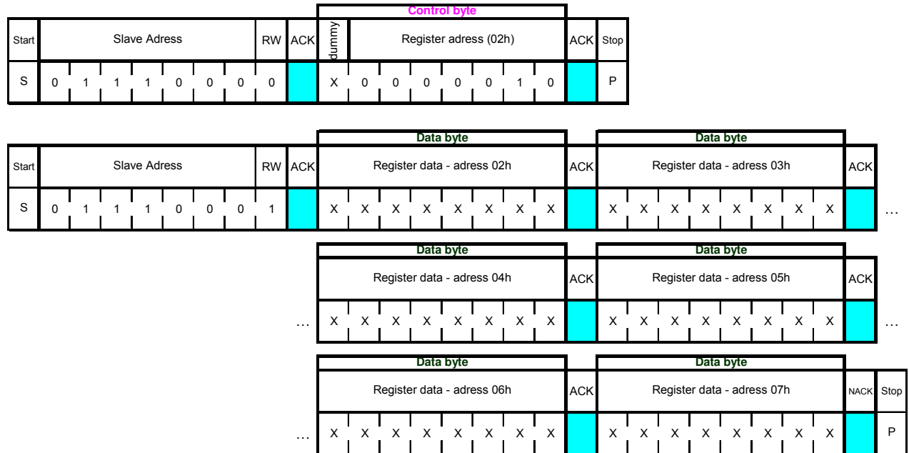
Figure 22: I 2 C multiple read protocol. Address register is first written to BMA150, the RW=0 (lowest acceleration data located at address 02h). I 2 C transfer is stopped and restarted with RW=1, address is automatically incremented and the 6 bytes can be sequentially read out.
