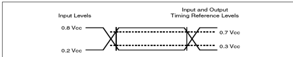
Figure 22. AC Measurement I/O Waveform
