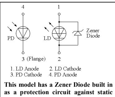
This model has a Zener Diode built in as a protection circuit against static electricity.
