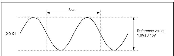
The amplitude changes by resistance, capacity which added outside or the difference of the device.
