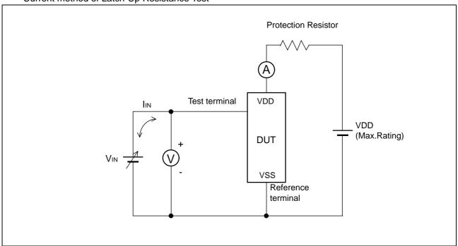
Note: The voltage  $V_{IN}$  is increased gradually and the current  $I_{IN}$  of 300 mA at maximum shall flow. Confirm the latch up does not occur under  $I_{IN} = \pm 300$  mA.
