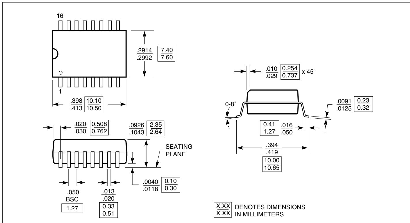
**Packaging Mechanical: 16-pin SOIC (W)**
