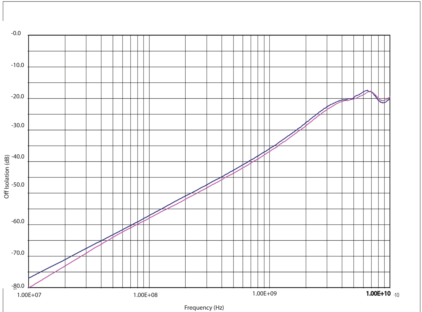
Fig 5. Off Isolation for SuperSpeed channels (Tx/Rx). Red is for path B and Blue is for path A
