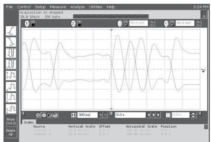
Data Waveforms, 2.5Gbps (left) & 5.0Gbps (right)
