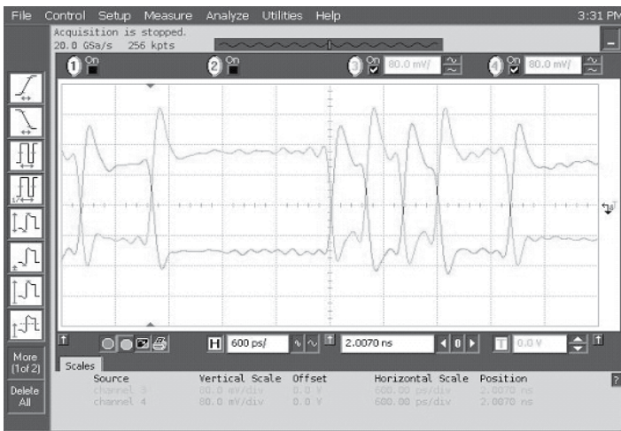
Data Waveforms, 2.5Gbps (left) & 5.0Gbps (right)
