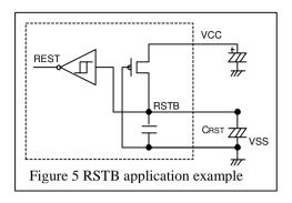
In case that the ZC signal disappears more than 3 seconds, the chip will restart the initialization operation. However, the restart initial time is always 40 seconds and cannot be extended by adding CRST to the RSTB pin as shown in Fig.5.
