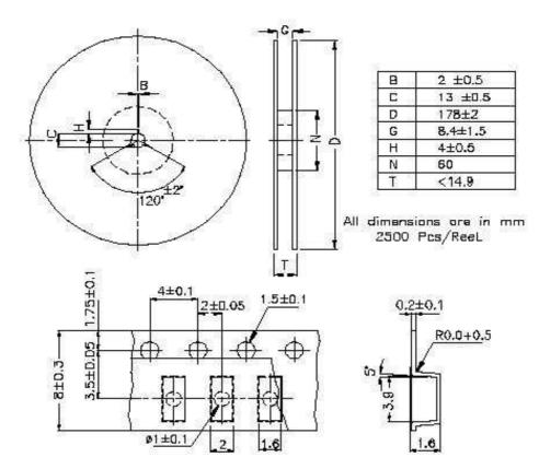
Accumulated pitch tolerance is  $\pm 0.2~\text{mm}$  over ID pitches 8-mm Carrier tape for Quadro MELF — LS34 PACKAGE All dimensions are in mm
