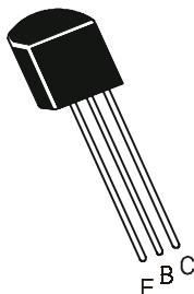
**Low Frequency Amplifier And High Frequency Oscillator.
