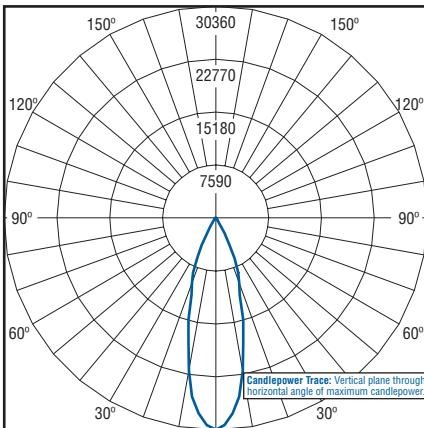
Independent Testing Laboratories certified test. Report No. ITL65016. Candlepower trace of 4000K, 60 LED 25° flood optic 304 series parking structure luminaire with 11,080 initial delivered lumens operating at 700mA. All published luminaire photometric testing performed to IESNA LM-79-08 standards.
