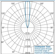
Independent Testing Laboratories certified test. Report No. ITL68860. Candlepower trace of 5700K, 2' (.6m) linear flood luminaire with 14 LEDs per foot. 15° flood optic with 5,080 initial delivered lumens operating at 700mA. All published luminaire photometric testing performed to IESNA LM-79-08 standards
