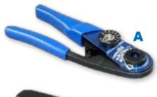
These crimp tools perform precision eight indent crimps for gas-tight wire terminations and excellent tensile strength. Adjustment wheel has 8 settings. Ratchet mechanism prevents improper crimps. Use with bayonet-type positioners. Check calibration with M22520/3 gages. Length is 6.75 inches, weight is approx. 10 oz.
