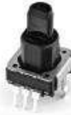
A typical rotary encoder
