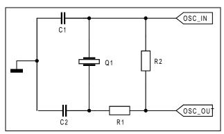
Figure 11: Oscillator Circuitry
