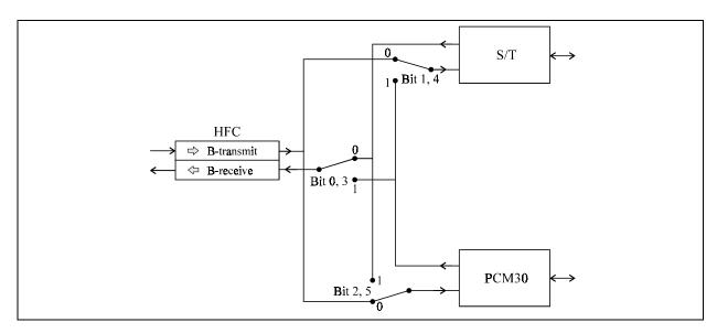
Figure 7: Function of the CONNECT register bits
