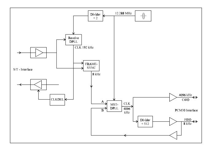
Figure 17: Clock synchronisation in TE-mode
