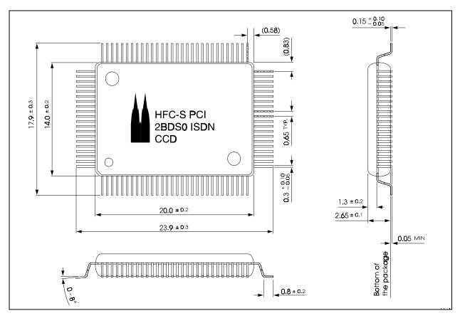
Figure 18: HFC-S PCI package dimensions
