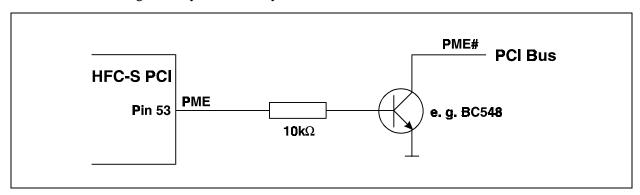
Figure 13: PME pin circuitry
