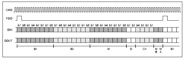
Figure 15: Single channel GCI format
