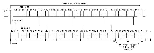
Figure 14: Frame structure at reference point S and T
