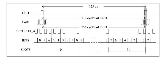
Figure 8: GCI/IOM2 bus clock and data alignment
