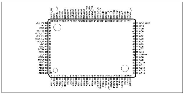
Figure 2: Pin Connection
