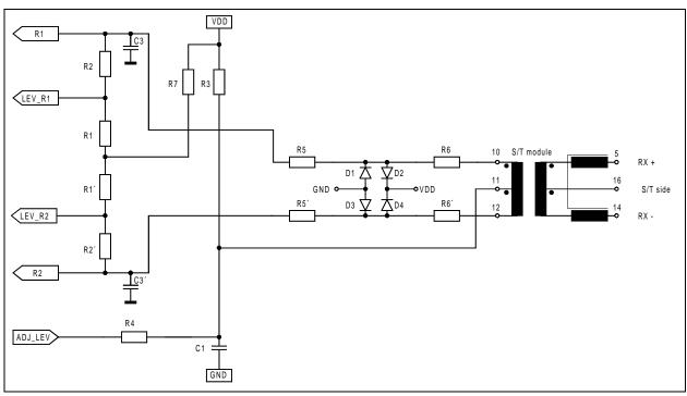
Figure 9: External receiver circuitry
