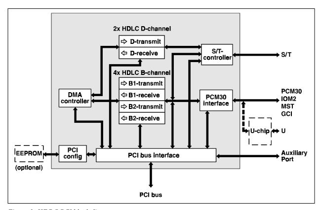
Figure 1: HFC-S PCI block diagram
