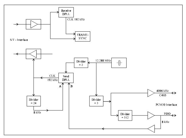
Figure 16: Clock synchronisation in NT-mode
