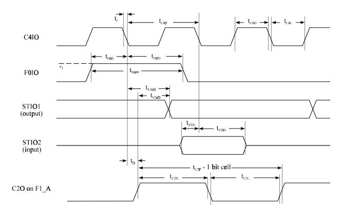
Timing diagram 1: GCI/IOM2 timing
