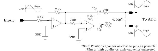
If decreasing component count is an important factor, and a decrease in performance specifications is acceptable, the AL1101G inputs may be driven unbalanced with a simple passive component conditioning circuit. The lowpass filter has fc = 72kHz.
