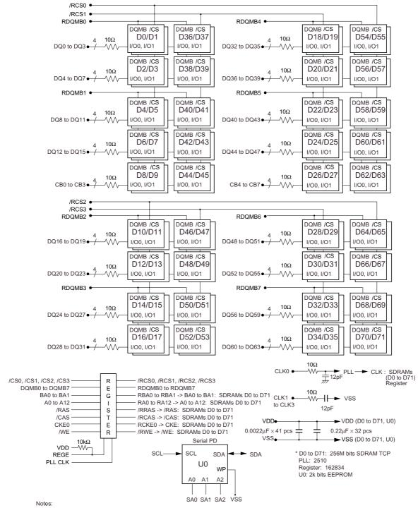
1. The SDA pull-up resistor is required due to the open-drain/open-collector output.
