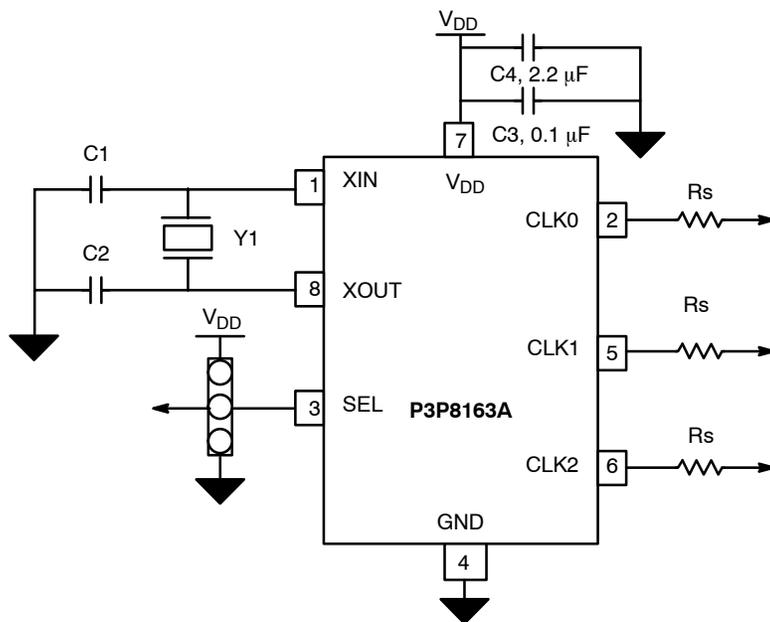
Rs = Trace Impedance of PCB – Output Impedance of Device (Z0)
