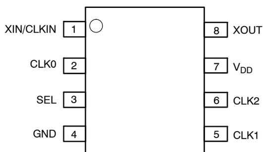
**Figure 2. Pin Configuration**
