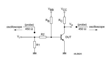
$$\begin{split} V_i &= 5 \; V; \; T = 500 \; \mu s; \; t_p = 10 \; \mu s; \; t_r = t_f \leq 3 \; ns. \\ R1 &= 56 \; \Omega; \; R2 = 2.5 \; k\Omega; \; R_B = 3.9 \; k\Omega; \; R_C = 270 \; \Omega. \end{split}$$
