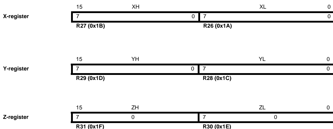
Figure 4-3. The X-, Y-, and Z-registers
